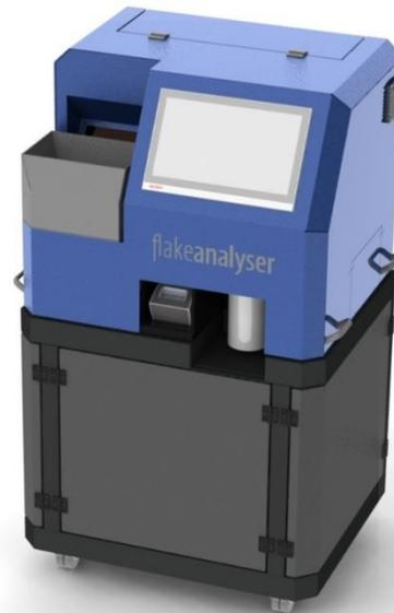
multi-sensor analysis device for quality control and material analysis of plastic regrinds
